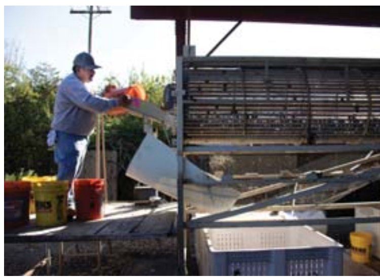
Chestnuts are poured into the sorting machine.
